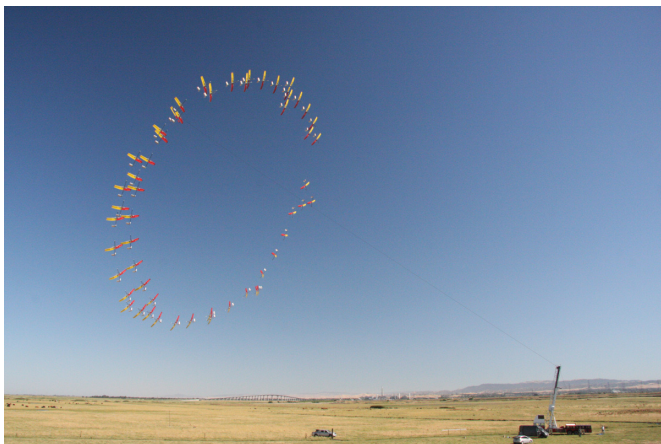
1. A composite of fifty-six images of a 10 kW prototype wing in flight under autonomous control.
